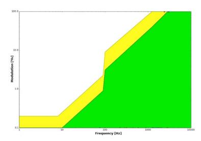
Thanks to the 4khz dimming frequency the MINI-1CV-CASAMBI allows to reduce the Flicker phenomenon.
